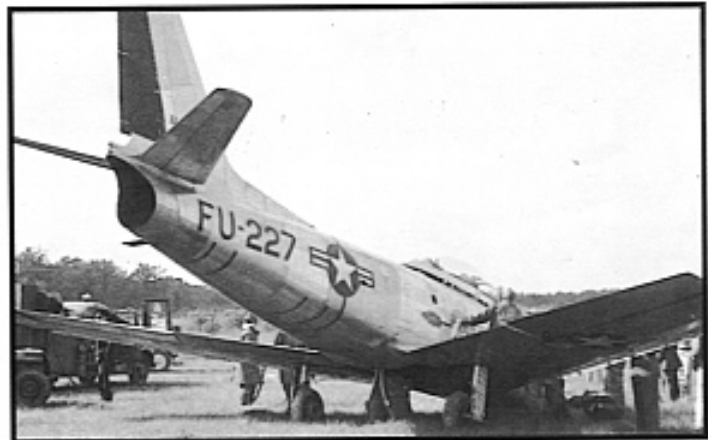
Lt. Dick Merian's 4th FIG F-86A lost all hydraulic power which didn't allow the nose gear to fully retract or extend and lock. Merian carefully landed the airplane and it slid to a stop on its nose.
