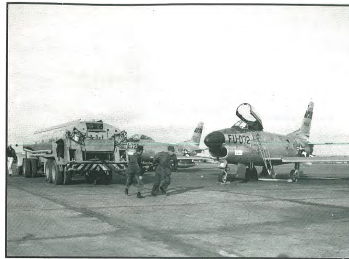
Tyndall AFB refueling crews pull hose to begin fueling an Interceptor Weapons School F-86D. Note the tail markings have been changed to the standard ATC tail logo with "TYNDALL" printed above the ATC badge. (credit - USAF)
