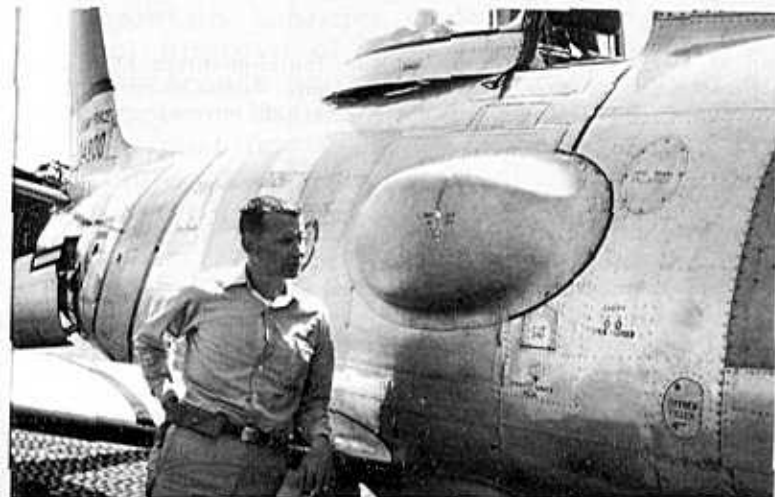
Ozzie Niedermann, North American Aviation Tech Rep at Kimpo in 1953, stands by one of the factory-built RF-86Fs. The bulged gun bay covered the camera body and film magazine of the vertically-mounted camera suite. (credit - Ozzie Niedermann)
