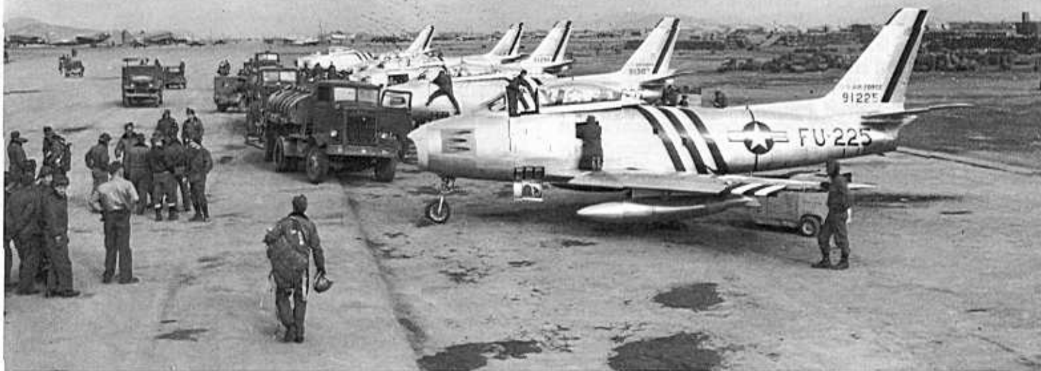
F-86As of the 4th FIG on the ramp at Suwon in the late Spring of 1951. The black and white stripes were added to all 4th FIG Sabres as a quick ID marking since the Sabre and MiG were similar in shape and size. The stripes were changed to black and yellow in 1952. (credit - USAF)
