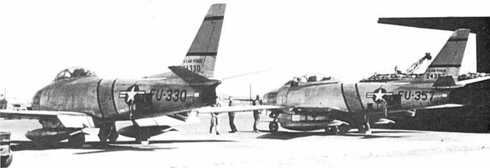
Two of the three RF-86F 'Haymaker' Sabres on the 67th TRW ramp at Kimpo in May 1953. All the Tsuiki-modified RF-86s had horizontally-mounted cameras that used a set of mirrors to reflect the image back to the camera lens. Although several of the RF-86Fs retained their gun ports, none were actually armed since gun vibration could knock the mirrors out of adjustment. Plus FEAF didn't want its recon pilots out chasing MiGs! (credit - Larry Davis)
