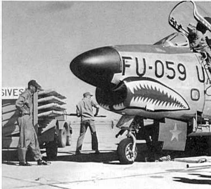
The single star on the nose door indicates the Sabre of BrigGen Agee, CO of 9th Air Division. Armourers are loading 2.75" FFAR rockets in the weapons bay on the ramp at Vincent AFB, Yuma, AZ in 1955. (credit - King Lotz)
