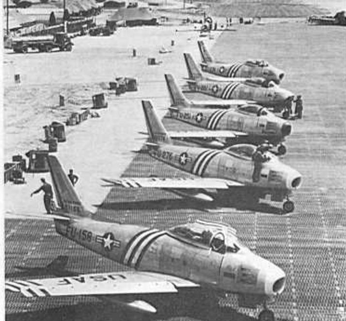
Five 335th FIS F-86As on the PSP parking ramp at Suwon in the summer of 1951. Suwon, 25 minutes from "MIG Alley", was so under-developed that landing Sabres were on the runway at the same time as aircraft taxiing back to their parking spots! (credit - Larry Davis)
