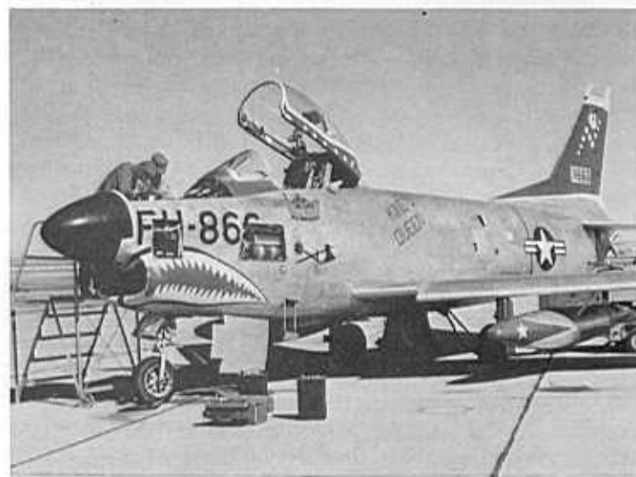
Two 498th FIS electronics specialists work on the Hughes E-4 Fire Control System of LT A.K. Lotz's "KING'S QUEEN", on the Yuma ramp in November 1955. (credit - King Lotz)
