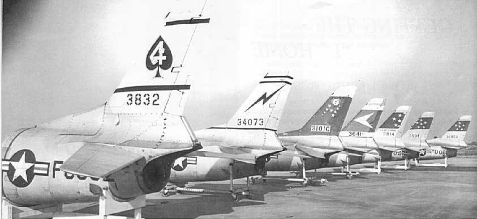
A lineup of F-86D aft fuselage sections at the Fresno North American Aviation conversion facility, await modification to F-86L. In addition to installation of the SAGE equipment, the aircraft were completely re-wired, and all necessary TCTOs were complied with. (credit - North American Aviation)
