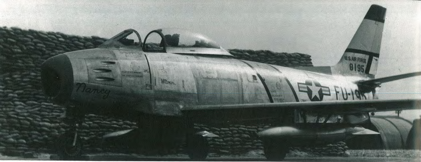
NANCY was flown by Lt Dick Burkhardt during the summer of 1952. Some of the RF-86As retained the .50 calibre machine guns, but firing them was discouraged due to vibration. (George McKay)
