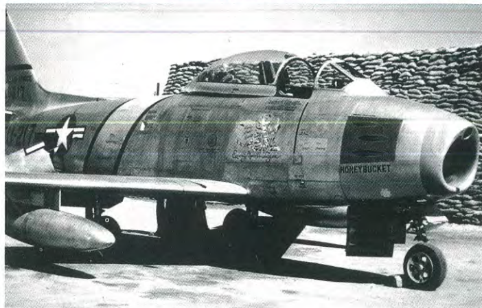
The #2 HONEYBUCKET RF-86A on the ramp at Kimpo after having the dicing camera installed in the upper nose. Note the lack of a fuselage fairing over the single camera in the right gun bay area. This aircraft was shot down by North Korean AAA, with Major Jack Williams, CO of the 15th TRS, being KIA. (R. Lamprecht)
