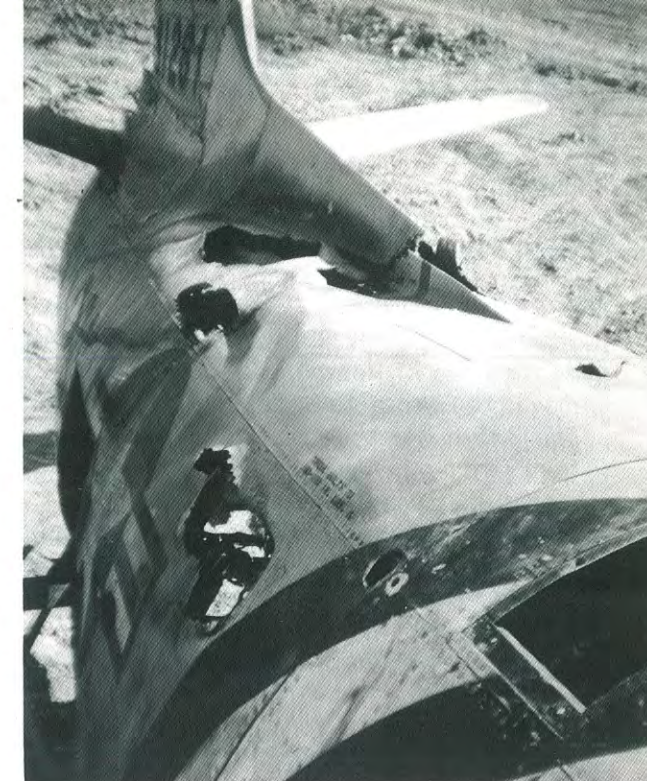
LtCol Glenn Eagleston - EAGLE - scratches his head in wonder as he surveys the damage to his gunbay from Casey Jones' 37mm cannon, which also put many holes in his aft fuselage. The 37mm hit also took out his throttle and most of his instruments. (Bruce Hinton, and John Henderson)
