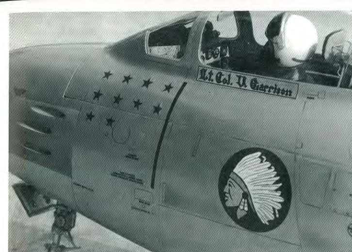
Looks real, doesn't it? The F-86F in the photos is actually a hand-built model with a wingspan of almost four feet, and weighing about eight pounds. The 1/2 cubic inch engine drives the model at well over 100 mph!
