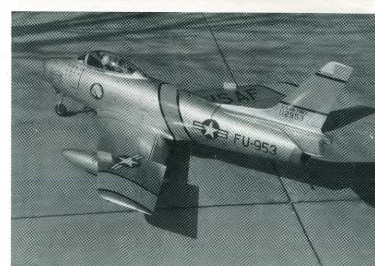
Looks real, doesn't it? The F-86F in the photos is actually a hand-built model with a wingspan of almost four feet, and weighing about eight pounds. The 1/2 cubic inch engine drives the model at well over 100 mph!
