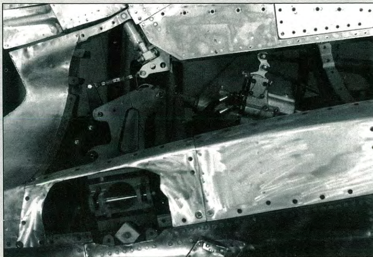
The longitudinal actuator and all vital castings in the rudder and fin had to be overhauled, inspected and tested. Note the massive size of the horizontal stabilizer mount.
