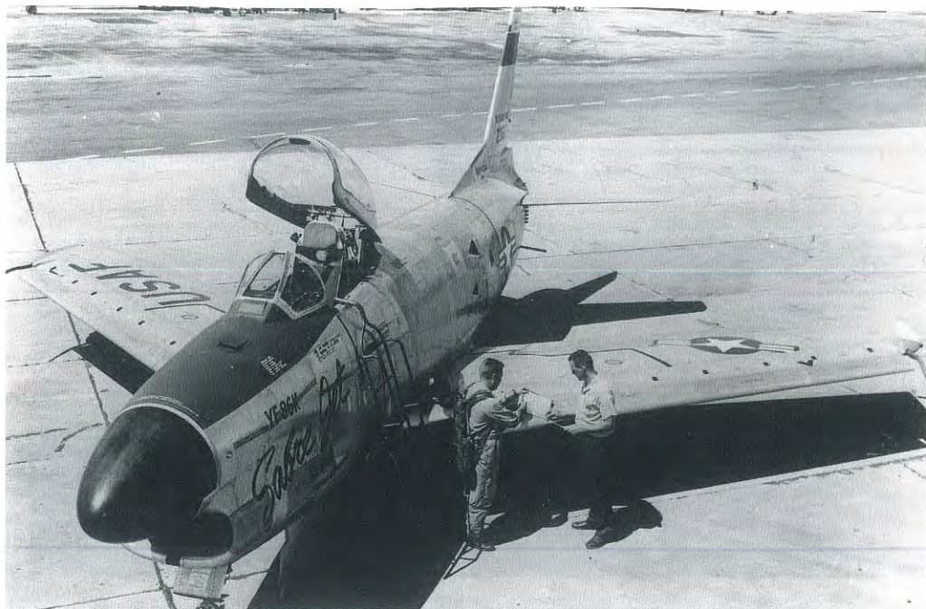
◀ Engineering Test Pilot Ray Norris talks with Flight Engineer Ray Richter prior to the first flight of the F-86K on 15 July 1954. The K model Sabre retained the all-weather radar of the D but substituted four 20mm cannon for the rocket armament. (credit – NAA)
