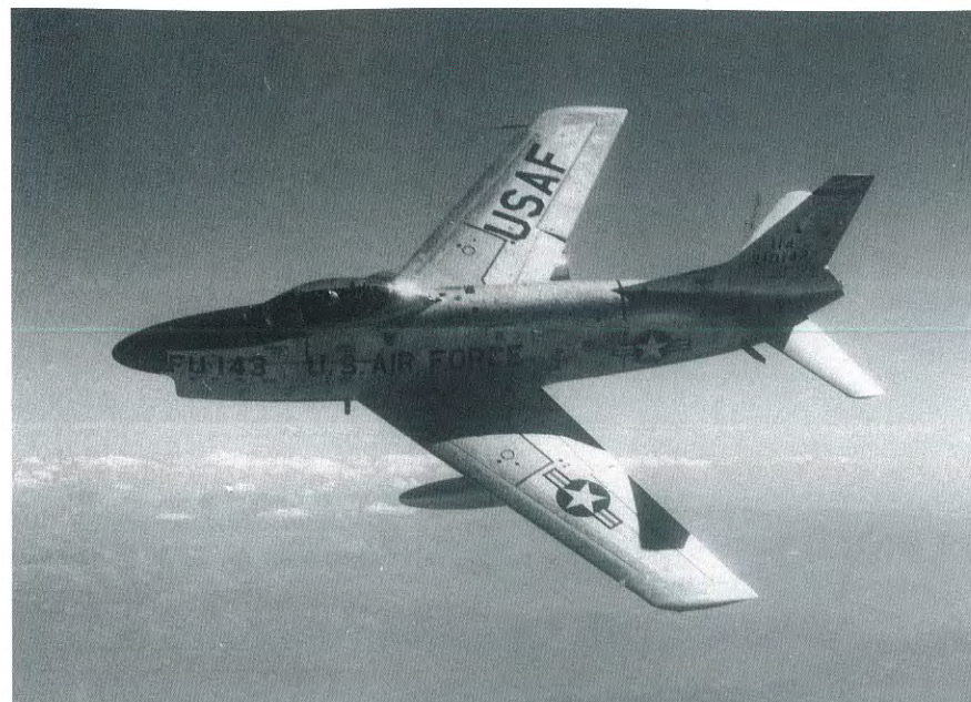
◀ The F-86L could be distinguished externally by seeing the SAGE antenna blade protruding from the fuselage in front of the wing. The other identifier was the longer and wider wing that was adapted from the day fighter types. (credit – NAA)
