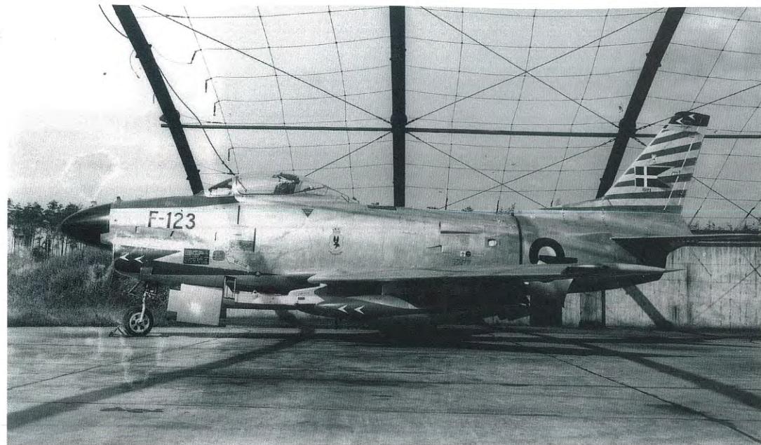
◀ An F-86D from no. 726 Eskadrilleskold based at Solingen, West Germany in April 1961, as part of the NATO air defense forces. Danish Air Force F-86Ds were modified to carry the AIM-9 Sidewinder missile after they were delivered. (credit – Merle Olmsted)
