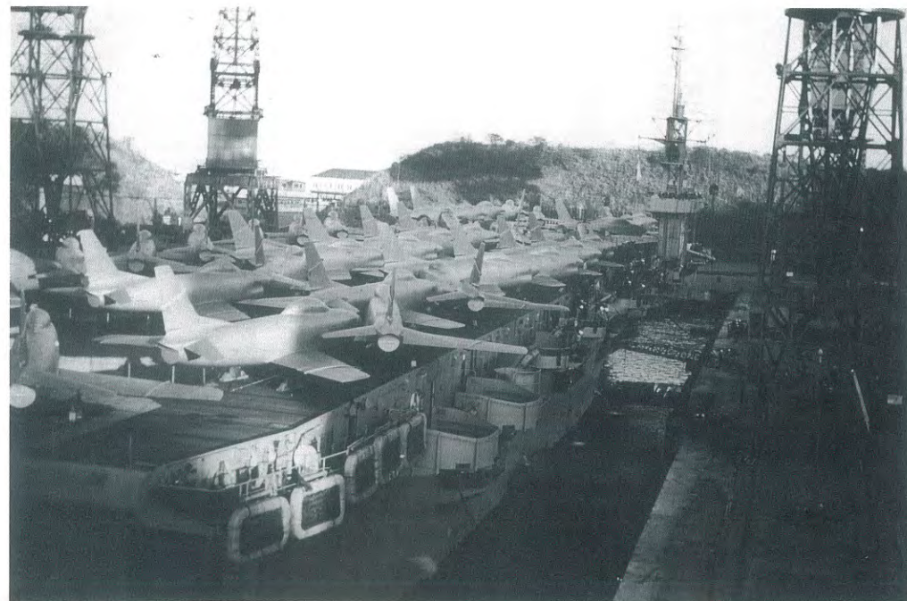
▶ Since no F-86 of any type was capable of inflight refueling, the US Navy brought the type to faraway shores like Japan. This is the USS Sitkoh Bay with a deck full of F-86D-45s bound for the 339th FIS at Chitose AB, on Northern Japan. (credit – Ed Levering)
