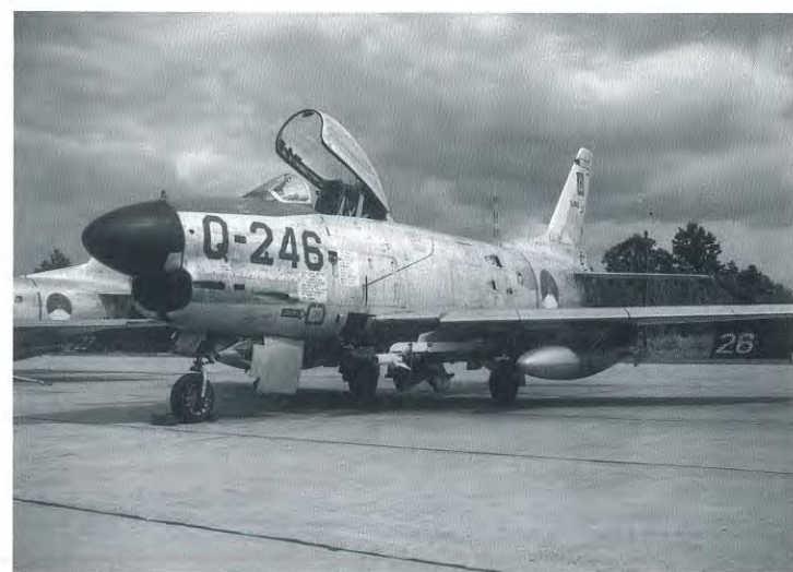
▲ This F-86K from the Netherlands Air Force, sits Ready Alert at Hahn AB, West Germany armed with a pair of AIM-9 Sidewinder air to air missiles. In addition to the Sidewinder armament mod, many Ks also had the extended wing added for better performance at altitude. (credit – RNAF)
