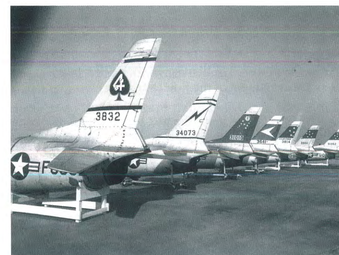
◀ During Project FOLLOW-ON that converted over 1000 F-86Ds to F-86L, the aft fuselage sections were removed and sent to Fresno for modification that included addition of the drag chute if it hadn't already been so equipped. The many squadron tail markings indicate that airplanes from throughout the D inventory were chosen for modification. (credit – NAA)
