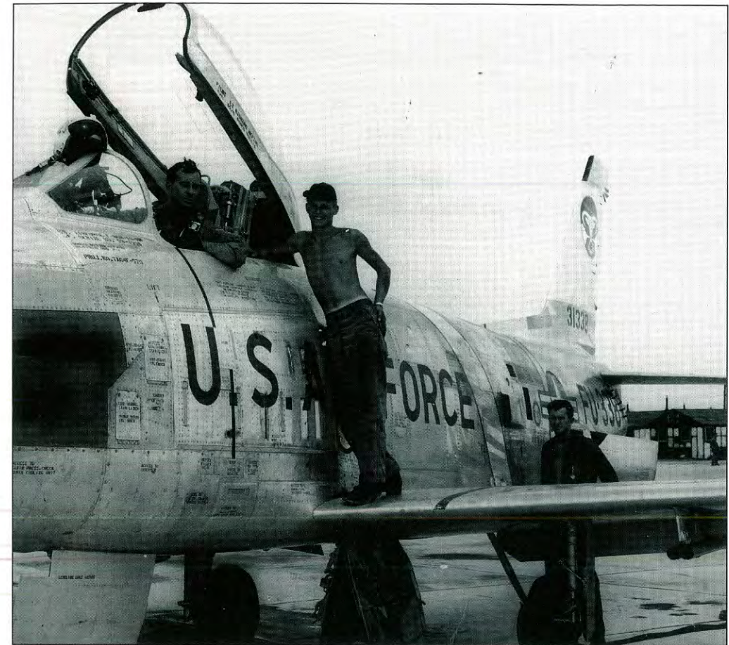
First Lieutenant Richard R. Hefton, who later retired as a Brigadier General, in the cockpit of a 34th Fighter-Day Squadron early F-86H from George Air Force Base in 1955. Note the lack of leading edge slats on this "H" Sabre. Photo courtesy of the U.S. Air Force via Dick Hefton.
