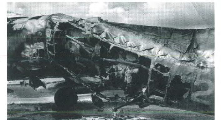
This 8th FBW F-86F suffered major damage when the engine exploded on the Suwon ramp in July 1953. The compressor failure took place during normal run-up on 14 July. Of special interest to historians is the fact that the airplane bears the logo "U.S. Air Force" on the fuselage, which was thought not to be carried until after the end of the Korean War. (credit - USAF)
