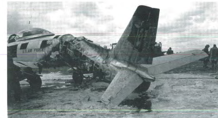
This 8th FBW F-86F suffered major damage when the engine exploded on the Suwon ramp in July 1953. The compressor failure took place during normal run-up on 14 July. Of special interest to historians is the fact that the airplane bears the logo "U.S. Air Force" on the fuselage, which was thought not to be carried until after the end of the Korean War. (credit - USAF)
