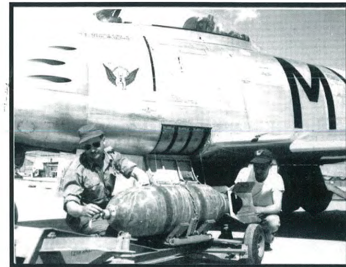
Armament technicians fuse a 1000 lb. bomb for installation on the underwing pylon 619-M. The aircraft was lost on 19 May 1953. (credit – SAAF)
