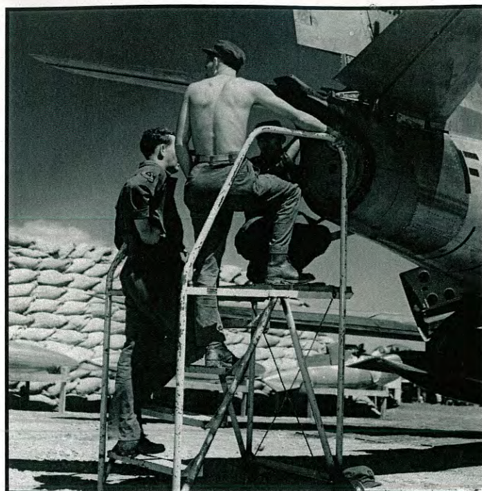
Crew chiefs remove the exhaust plug from one of the new F-86Es that equipped the 51st FIG in October 1951. Some pilots were transferred from the 4th FIG at Kimpo, to the 51st FIG at Suwon when the 51st re-equipped with Sabres. Lt. Frank Robison was one of those pilots. (credit- USAF)
