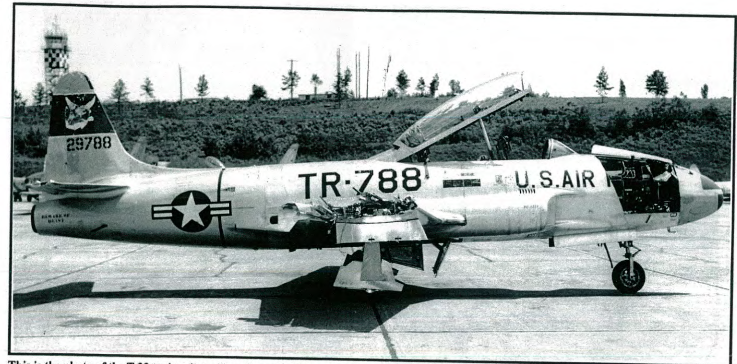
This is the photo of the T-33 trainer/target tug flown by John Johnston and reported in Sabrejet Classics vol. 20-3. The collision took off about 4 feet of wing but Johnston brought it back to Stewart for a safe landing. (credit - John Johnston)
