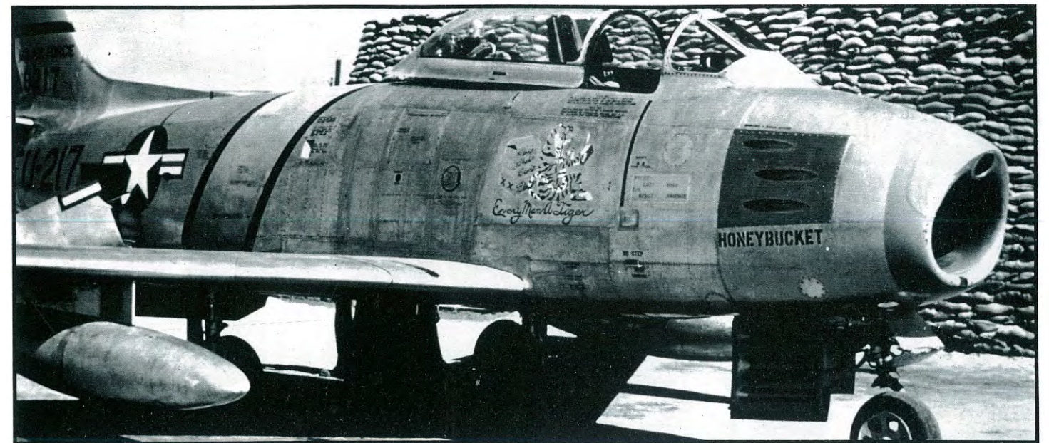
RF-86A #48-217 is the Ashtray Sabre that Lt. Fosdick flew on his 97th mission. The Sabre was lost on a later mission with the 15th TRS Commander, Major Jack Williams, listed KIA. Note the modified upper intake housing the dicing camera. (credit - Robert Lamprecht)
