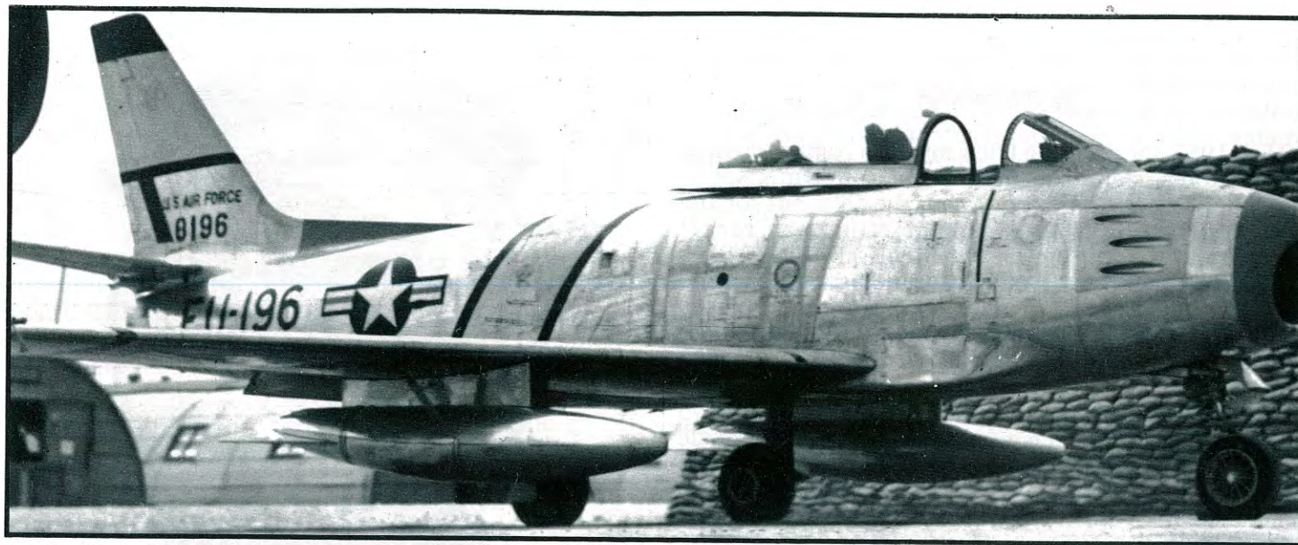
A pair of 15th TRS RF-86As in the revetments at Kimpo in 1952. The RF-86A Ashtray aircraft had a single camera mounted in the underside of the right fuselage, and were converted from ex-4th FIG F86As. The Ashtray Sabres were painted identical to 4th FIG Sabres. (credit - George McKay)
