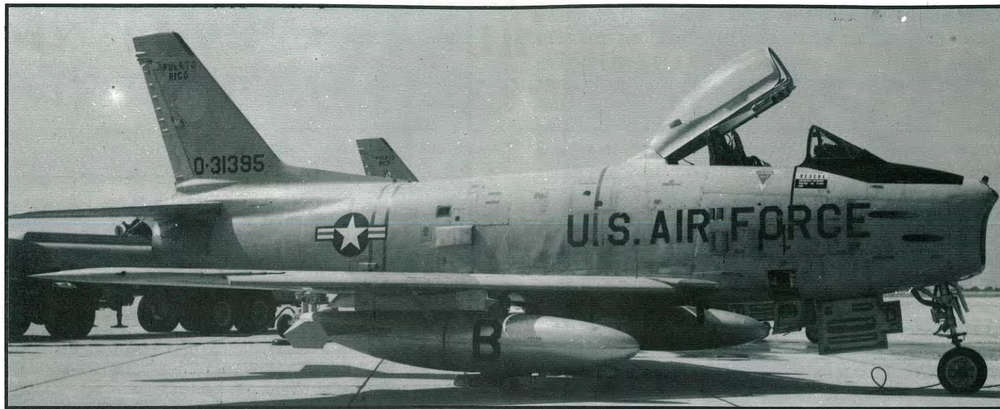
A PRANG F-86H at Isla Verde, wears the overall grey paint adopted by USAF for anti-corrosion in the mid-1960s. The 198th TFS converted from the F-86H to F-104Cs in July 1967. (credit - Larry Davis coll.)
