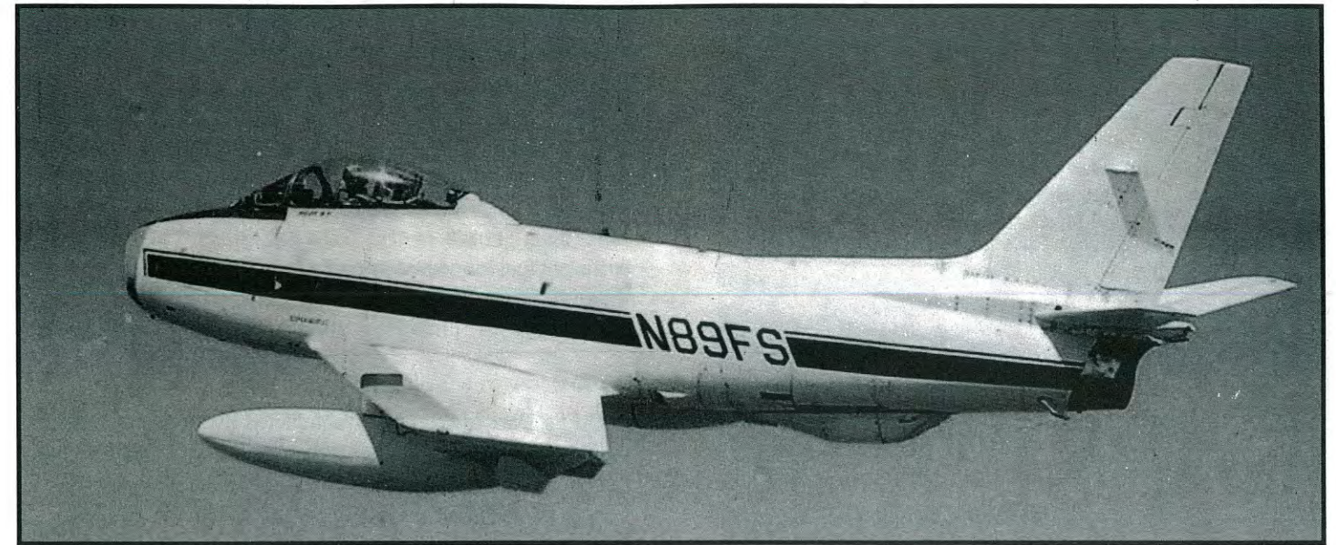
An FSI Sabre Mk 6 with the centerline Dart Tow package. (credit - JR Alley)
