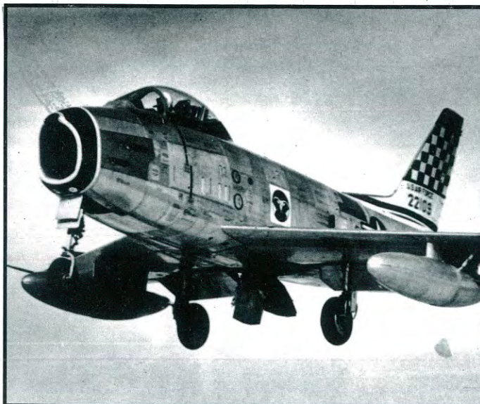
An F-86H-5 from the 34th FDS, takes off from George AFB in 1956. All F-86Hs except the prototypes, were built at the North American plant in Columbus, Ohio. The wing fence is clearly seen. (credit - USAF)
