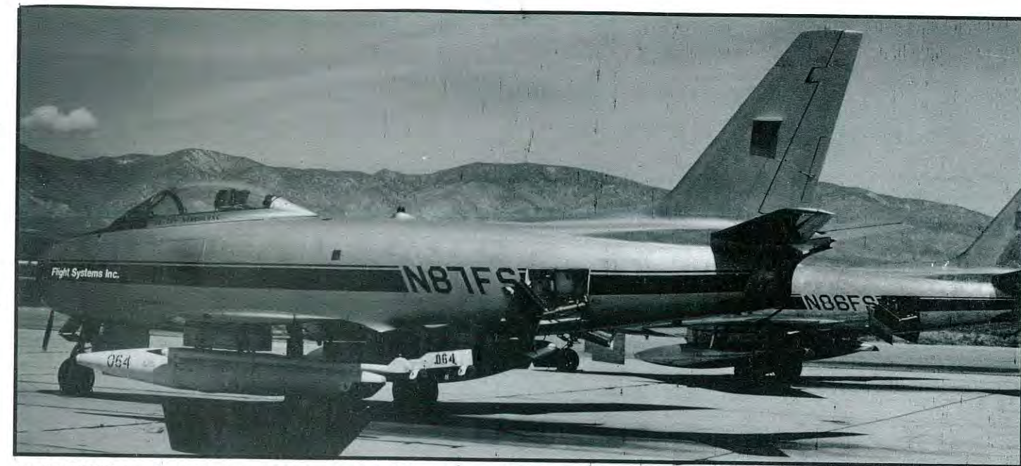
A pair of FSI Sabre 6s on the ramp at Mojave in May 1982. The near aircraft has the A/A37U-15 Tow Reel but not the Dart. (credit - Bob Shane)
