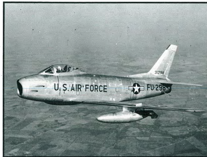
An F-86H-10 makes a test flight over Ohio in 1956. The H-10 had the four 20mm cannon introduced with the H-5, but retained the hard wing as all previous variants. (credit - NAA)
