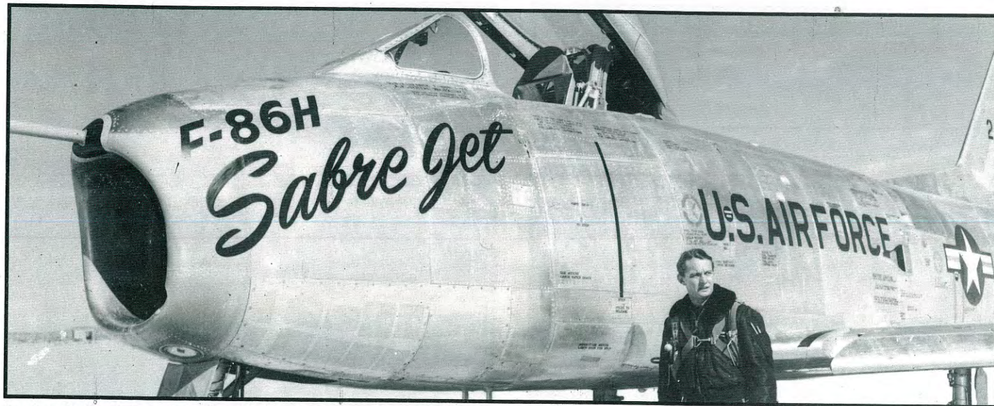
Joe Lynch, North American Test Pilot, stands next to the first F-86H, #52-1975, prior to the first flight on 30 April 1953. The first two aircraft built had the original short chord/short span/slatted wing used on the F-86A/E/early F, with no armament. (credit - NAA)
