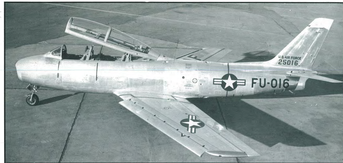
The TF-86F used the same wing as the F-86E/F, which was moved forward 8 inches to reposition the center of gravity. The wing was the early short chord, short span wing with leading edge slats. (credit - NAA)
