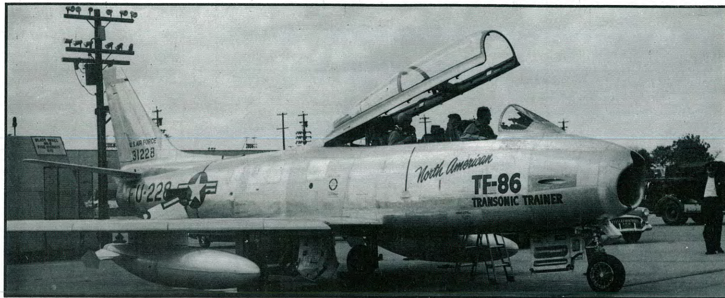
After the first prototype crashed and was destroyed in March 1954, North American built a second TF-86F prototype, serial 53-1228. It differed from the first only by having a pair of .50 caliber machine guns in the nose. (credit - NAA)
