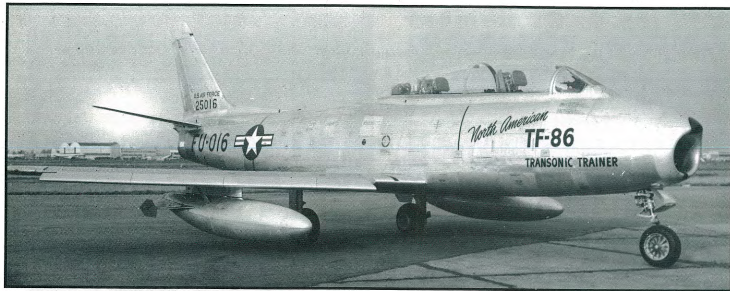
The TF-86F prototype, serial 52-5016, in January 1954. The TF-86F was slated to be the first transonic trainer in the Air Force. However, the TF-100C, with supersonic capabilities, won the 'competition'. The TF-86F was almost 6 feet longer than a standard F-86F. (credit - NAA)
