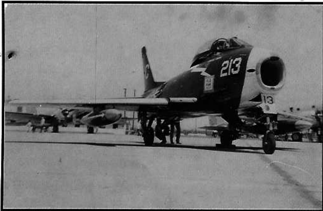
An FJ-3 from VF-33 during an air show at New Castle Airport in 1956. The enlarged intake was needed for maximum thrust from the J65 engine. The redesigned nose gear that was needed for launches from the carrier, is clearly seen. (credit - Larry Davis collection)
