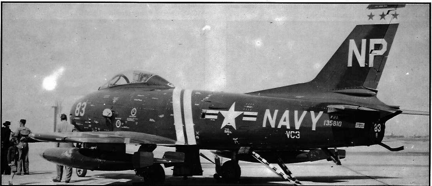
An FJ-3 from VC-3 shows the tail hook and bumper assembly needed for carrier landings. Initially, all Navy FJ-3s were delivered in standard Navy Blue paint. Note the 200 gallon streamlined drop tanks. (credit - Wm. T Larkins)
