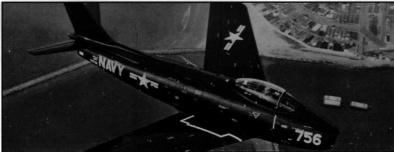
An XFJ-2B Fury over Long Beach in 1952. The XFJ-2B was the first swept wing Fury to be delivered, and the first to have four Colt Mk.12 20mm cannons as armament. The XFJ-2 and production FJ-2s were basically a 'navalized' version of the F-86E with the all-flying tail and J47 powerplant. (credit - NAA)
