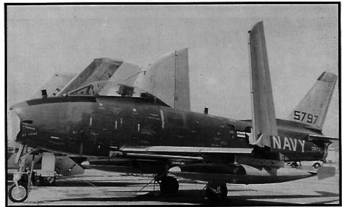
An FJ-3D2 drone controller from VU-3 showing how the wing folded right at the flap/aileron panel line. (credit - Wm. T. Larkins)
