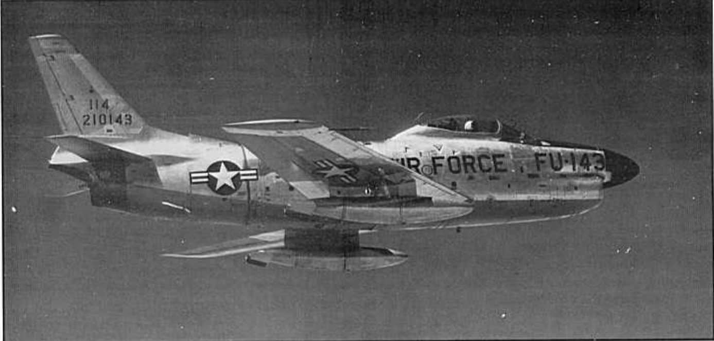
A 'new' F-86L-50 during the delivery flight in 1957. The extended wings installed on the L can be seen; with the SAGE antenna stub just visible under the forward fuselage. Many of the later L conversions had the underside of the fuselage painted Gloss Grey for corrosion control. (credit - NAA)
