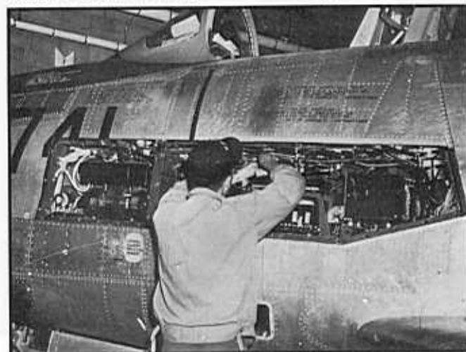
A North American employee makes adjustments in the electronics bay of one of the F-86Ds that were being converted to L. Under Project FOLLOW-ON, all the wiring was removed and replaced. (credit - NAA)
