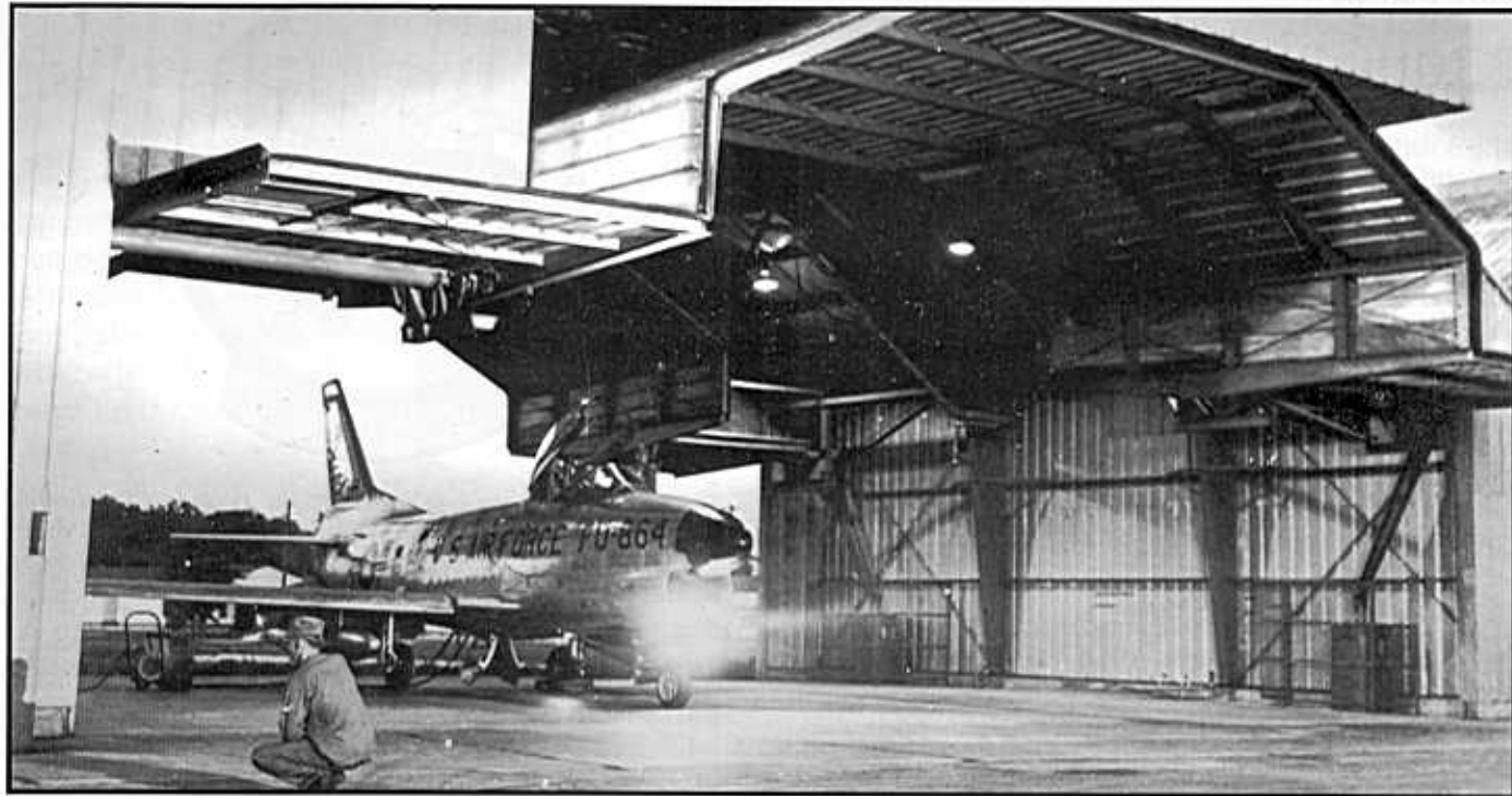
An 11th FIS F-86D in the alert barn at Duluth MAP in the 1950s. 'Barns' such as these were required by any squadron operating in cold weather areas along the northern borders. (credit - USAF)
