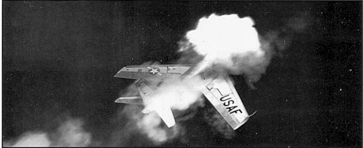
An F-86D lets loose with a volley of rockets over the California test range. The F-86D was the first one man interceptor and also used the radical idea of an all-rocket armament. The 2.75" Mighty Mouse rockets could be fired all at once or in various sequences. (credit - NAA)
