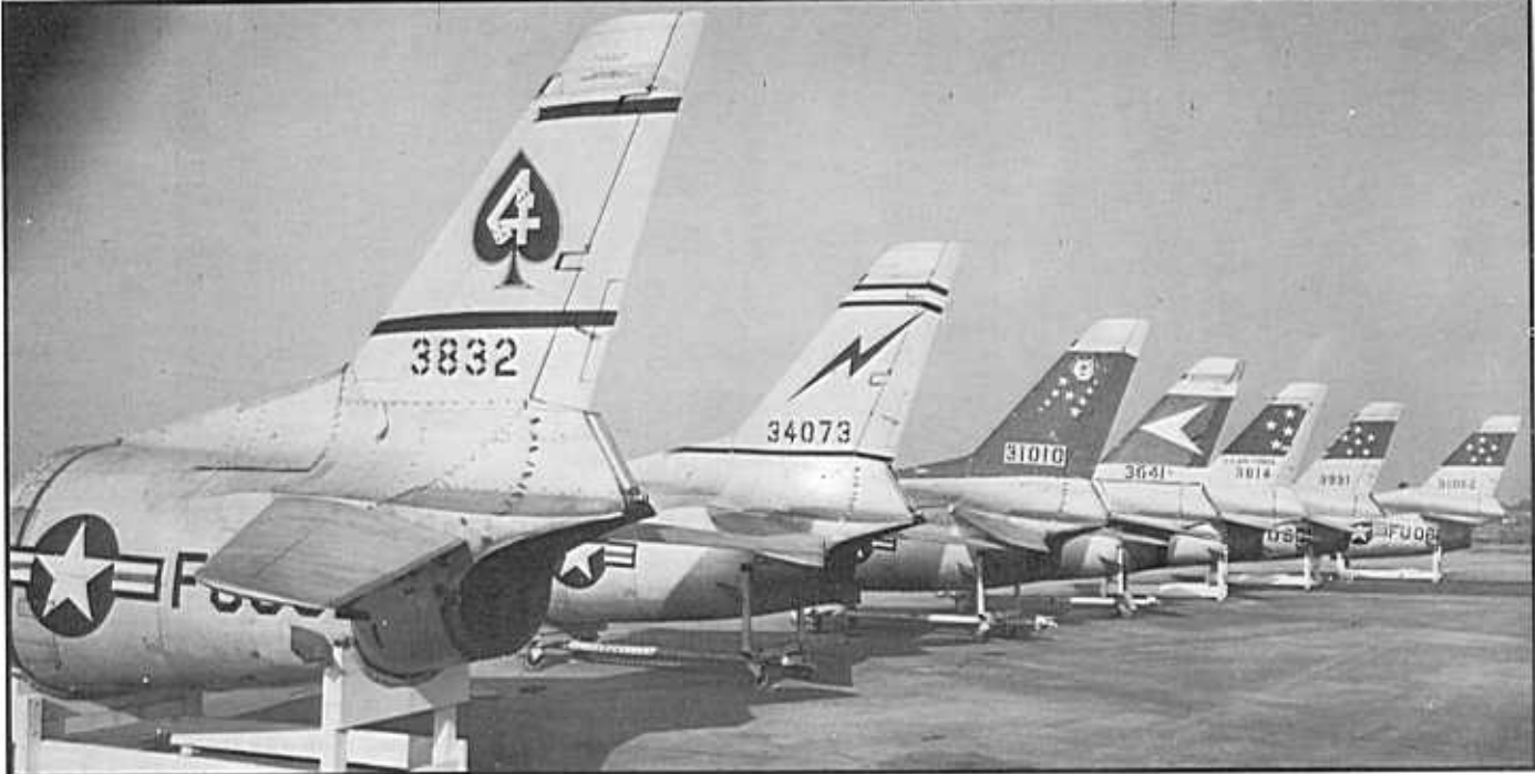
A lineup of aft fuselage sections awaiting FOLLOW-ON conversion at the North American plant in Fresno, CA. All the aircraft were drawn from active squadrons and brought up to the latest D standard including installation of the J47-33 engine. From L-R, 47th FIS, 31st FIS, 498th FIS, 329th FIS, 330th FIS, and two from the 332nd FIS (credit - NAA)
