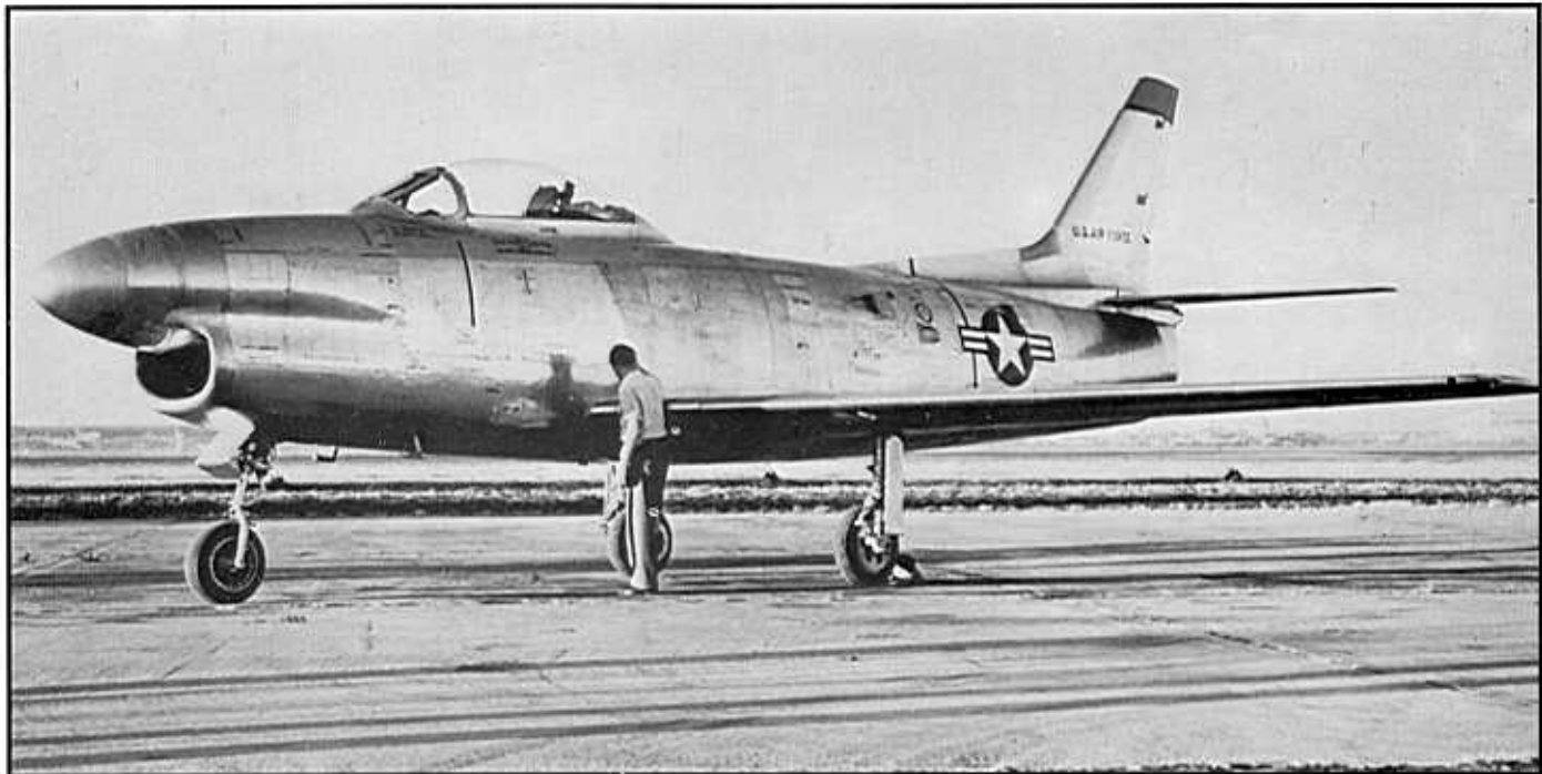
Rollout of the YF-86D interceptor came in early December 1949, with the first flight taking place on 22 December 1949. Eagle-eyed observers will note that the YF-86D retains several features of the F-86A including the V-shaped windscreen. (credit - NAA)
