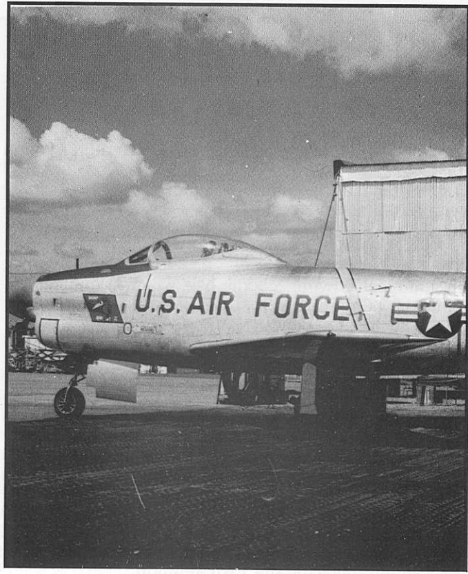
"Womp Bird II", a 26th FIS F-86D, is undergoing some work on the troublesome afterburner of the J47-GE-33 engine. (credit - Merle Olmsted)
