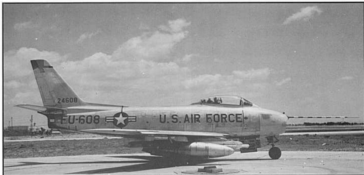
F-86F #52-4608 was pulled from the line and modified with the addition of a Rocketdyne AR2-3 rocket engine under the fuselage, whereupon the Sabre was redesignated JF-86F. Several North American test pilots flew the rocket-assisted Sabre including J.O. Roberts, Jim Brooks, and Jay Hanks. (credit - NAA)
