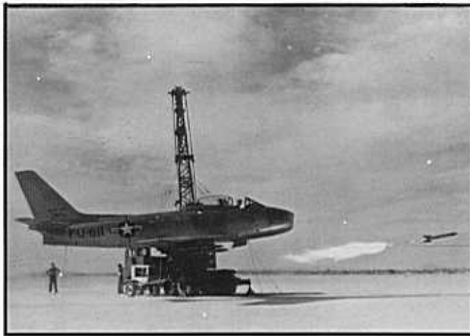
Following the record breaking flights of 15 September 1948, #47-611 returned to the normal business of testing new systems, including launch tests of 5" HVAR rockets. (credit - USAFM)
