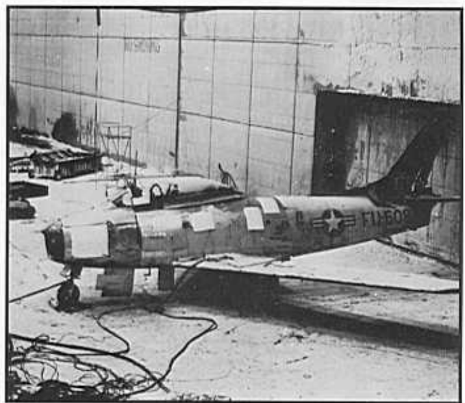
Following the record flights at Cleveland, the Sabre returned to its duties as a flight test aircraft. It is seen here later that summer, inside the Climatic Hangar at Eglin AFB where the temperature was -65^{\circ} F. (credit - USAF)
