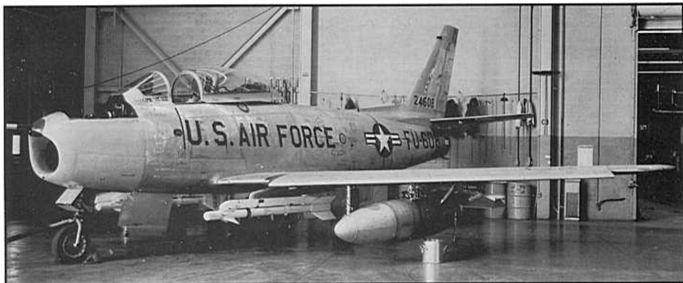
The JF-86F in a hangar at Edwards AFB in the Spring of 1960 after being modified to launch the AIM-9B Sidewinder missile. The 200 gallon underwing tanks held the hydrogen peroxide oxidizer. Reliability of the JF-86F/AR2-3 approached 100%, but supersonic interceptors like the F-104 Starfighter made the combination obsolete. (credit - NAA)
