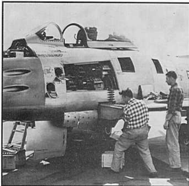
Robbie Robertson, NAA Armament Engineer, loads a 20mm ammunition canister into a GUN-VAL F-86F prior to delivery of the airplanes to the Eglin AFB Armament Test Center. Robbie personally made many of the hardware improvements on the T-160 system. Note the elongated and thinner gun bay. (credit - NAA)
