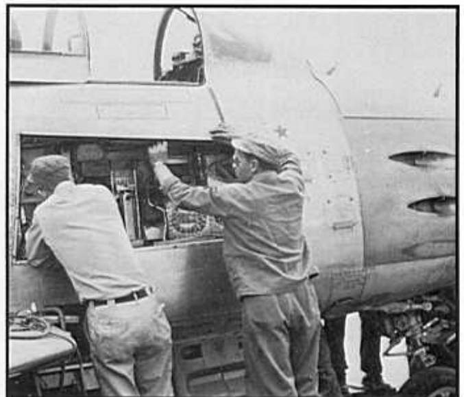
GUN-VAL armorers work on one of the 20mm cannons in the restricted area of the 335th FIS flightline. Note the deflector has already been welded into the gun port. Paul Peterson hand carried the deflector kits to Korea and had them installed on the seven remaining GUN-VAL Sabres at K-14. (credit - Paul Peterson)
