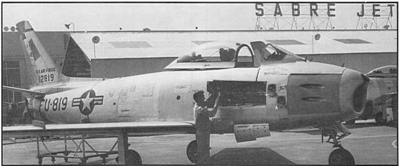
Rollout photo of an F-86F-2 GUN-VAL Sabre at North American Aviation's Inglewood plant. All GUN-VAL Sabres had the '6-3 hard wing' in addition to the 20mm cannon armament. Note the holes drilled in the ammo bay doors to relieve gun gas buildup. (credit - NAA)
