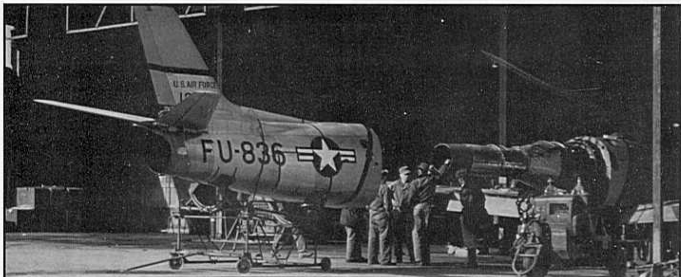
Although armament maintenance and support was performed on the 335th FIS restricted flight line, normal maintenance of all other systems, including the engine and flight controls, was performed in the maintenance shops at K-14. GUN-VAL Sabre #52-2836 is about to receive a new J47 engine.. (credit - Norman Green)
