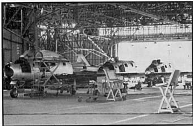
Inside the Air Asla shops at Tainan in 1957. One of the operations performed at Air Asla was bringing the F-86Fs up to the latest standards, including installation of the 6-3 wing as well as the "F-40" wing extension. Installation of AIM-9 Sidewinder launch capabilities was also done at Air Asla. (credit - Sid Yahn)
