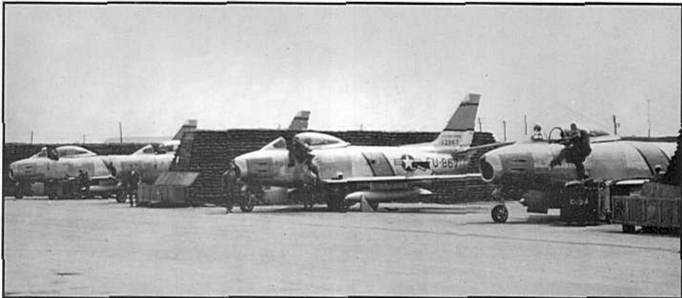
Project GUN-VAL pilots climb into the cockpit of four of the 20mm armed F-86Fs at Kimpo in Spring 1953. Eight GUN-VAL Sabres were sent to Korea for combat evaluation, and were assigned to the 335th FIS at Kimpo. Two were lost to inflight accidents involving gun gas ingestion. (credit - Paul Peterson)
