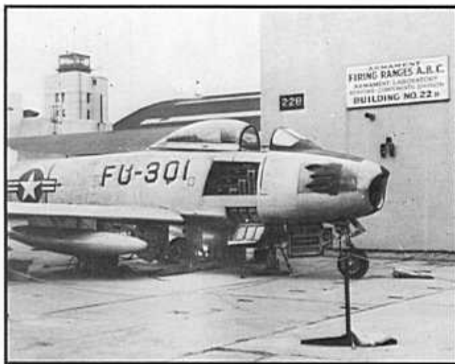
F-86A #49-1301, the wing tip tank test airplane, was delivered to the Wright Air Development Center where it was used to test various armament loads. (credit - David Menard collection)
