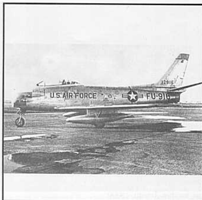
The F-86F-3 was a test of the Oerlikon 20mm cannon installation in an F-86F air frame. Similar in design to the T-160 installation, the Oerlikon guns were much larger and protruded through the fuselage. The Oerlikon installation was scrapped. (credit - John Henderson collection)
