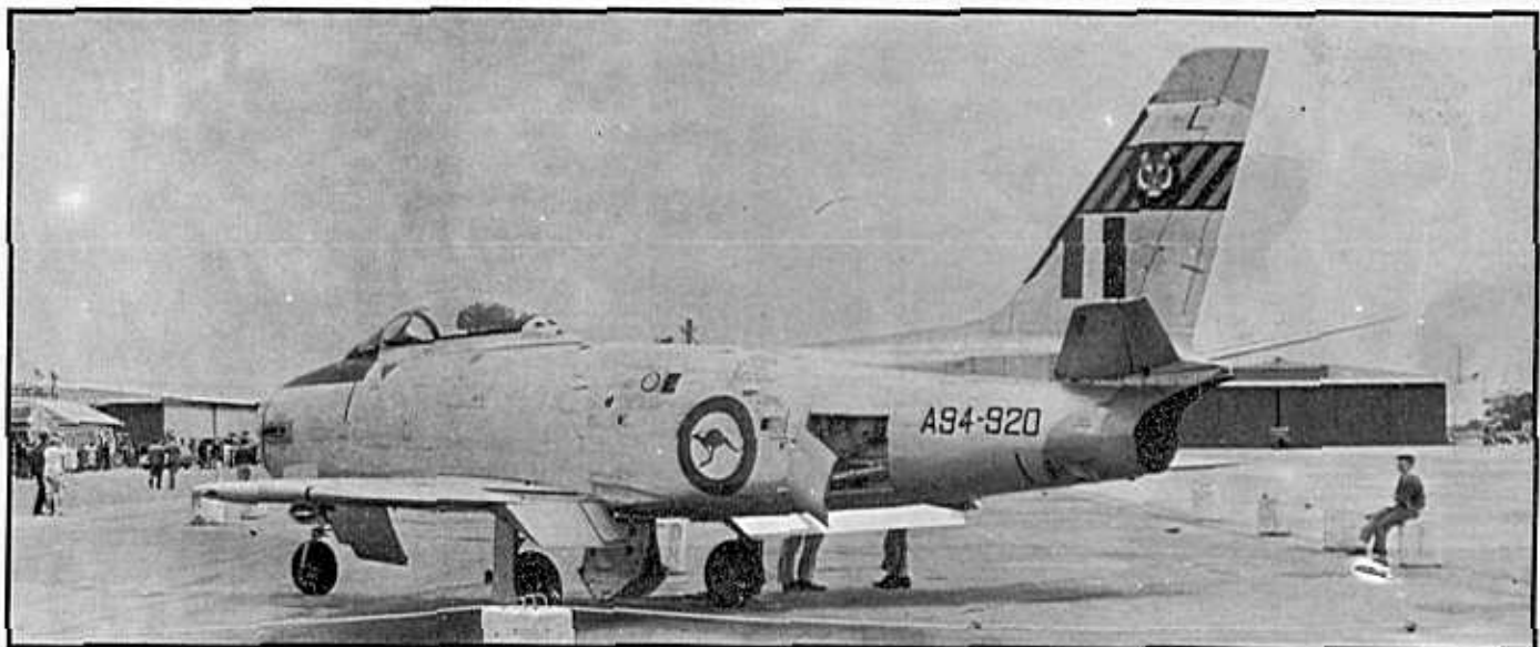
All CAC Sabres were brought up to Mk. 32 standard in 1960s, including addition of underwing launch rails to carry and fire the AIM-9 Sidewinder missile. (credit - Mike Fox)
