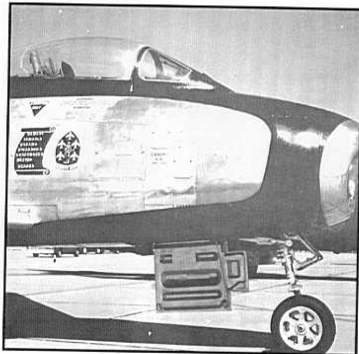
Top Left: MinuteMen F-86F-2 Sabre on the ramp at Buckley ANG Base. Note that the Sabre has only two gun ports due to the fact that the F-2s were armed with four 20mm cannon originally. (credit - Chub Trainor)
