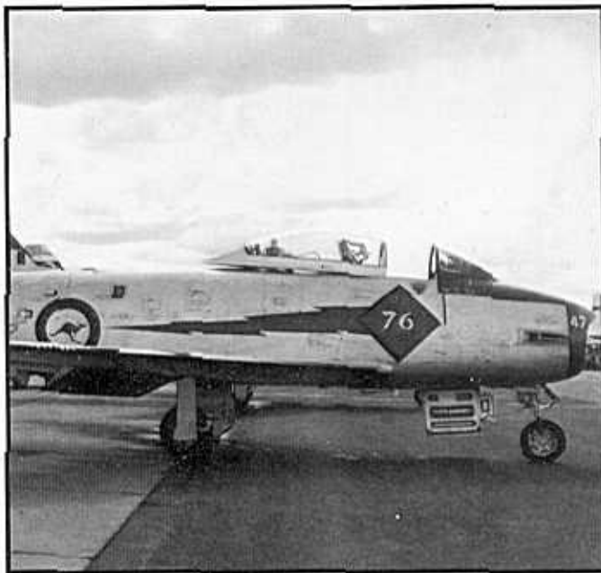
A CA-27 Sabre from No. 75 Squadron, on the ramp at Williamstown in the mid-1960s. Note that the Sabres have been painted in overall silver lacquer for corrosion control. (credit - J.A. Vella)
