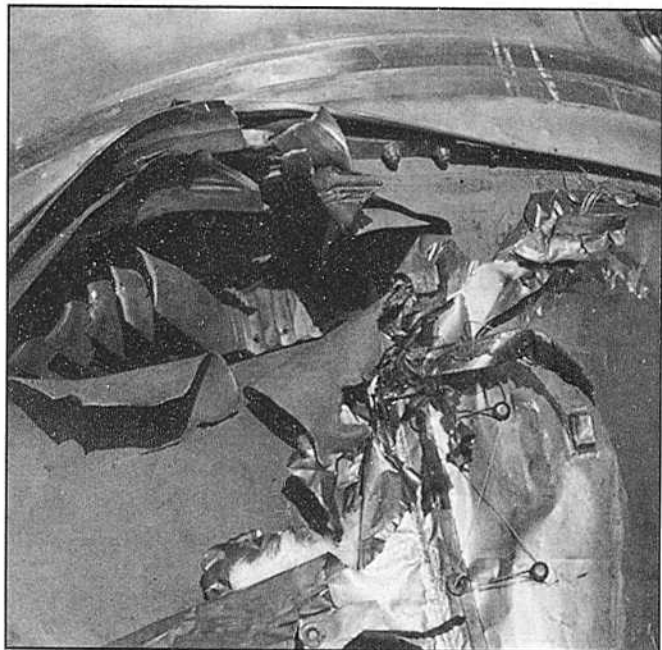
The engine compressor in Bob Matasick's F-86F showing the damage caused when five compressor blades cut loose. (credit - Bob Matasick)
