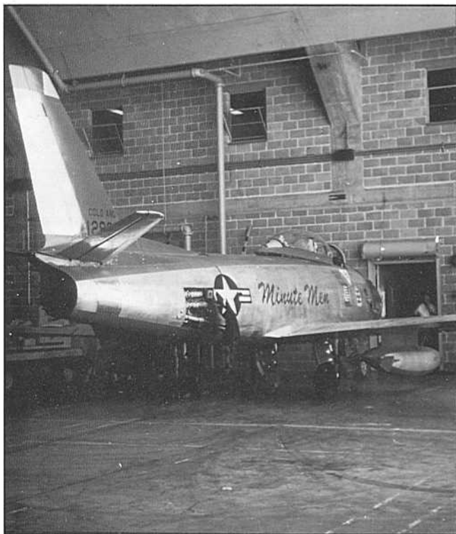
A "Minute Men" F-86F-2 in the maintenance shops at Buckley in 1958. The F-86F-2s that the team flew, had been experimentally fitted with T-160 (M39) 20mm cannons and combat tested in Korea with members of the 4th FIG. (credit - Pete Garremone)
