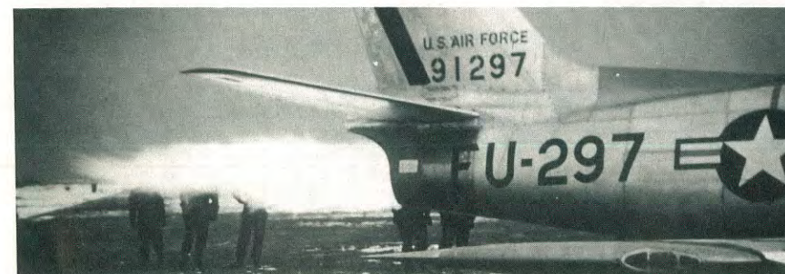
A hot start on a 4th FG F-86A-5. Major Billy Hovde aborted his start, but then restarted too quickly. The result was a fire blast out the tail section. Fortunately, no injury or damage resulted.
