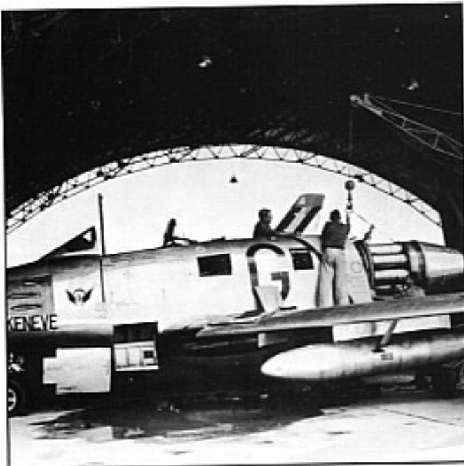
613 - G (52-4327) gets a new engine at the Tsuiki, Japan, REMCO facility in April 1953. 'G for George' was written off on 21 April. (credit - R.L. Ward)
