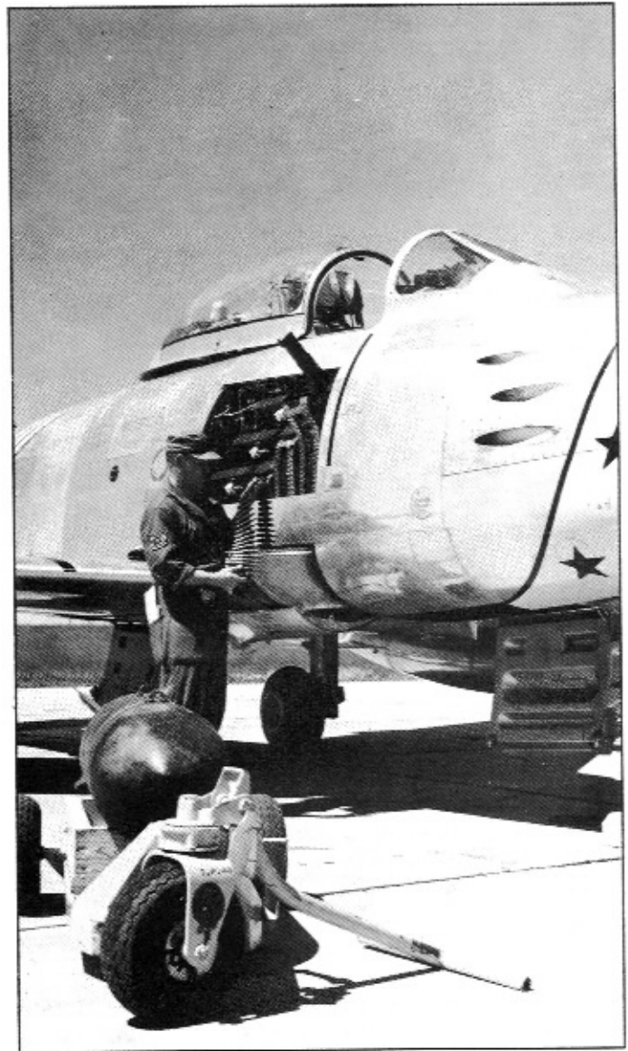
An armorer loads a belt of .50 caliber ammo into the ammo box of a 531st FBS Sabre on the ramp at Wheelus AB in the Summer of 1955. Live munitions could be used on the Wheelus gunnery range. The 500# bomb will be loaded under the wing on one of two available munition pylons. (credit - Larry Davis Collection)
