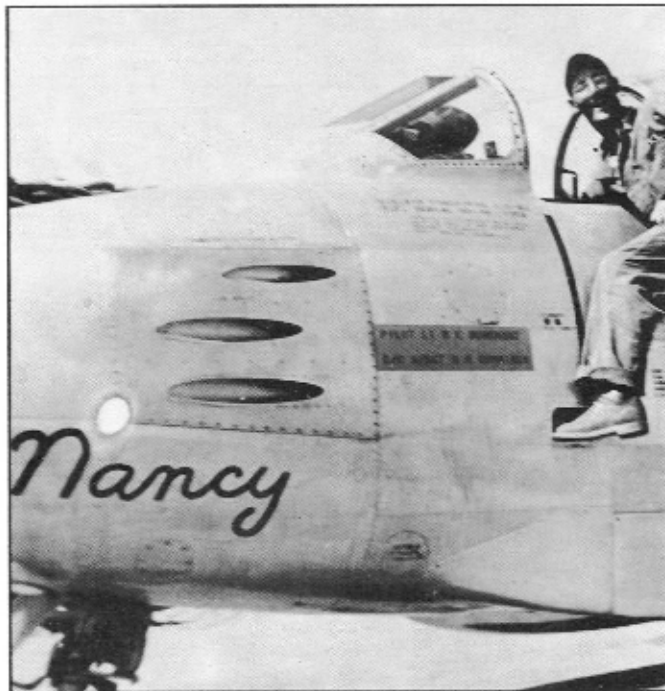
S/SGT Cummings smiles for the camera as he checks the cockpit of Lt. Bob Burkhart's RF-86A, #48-195 at K-14 in the Summer of 1952. Some RF-86As, and even a few of the early RF-86Fs, had the upper pair of .50 Caliber guns operational. (credit - Bill Coffey)
