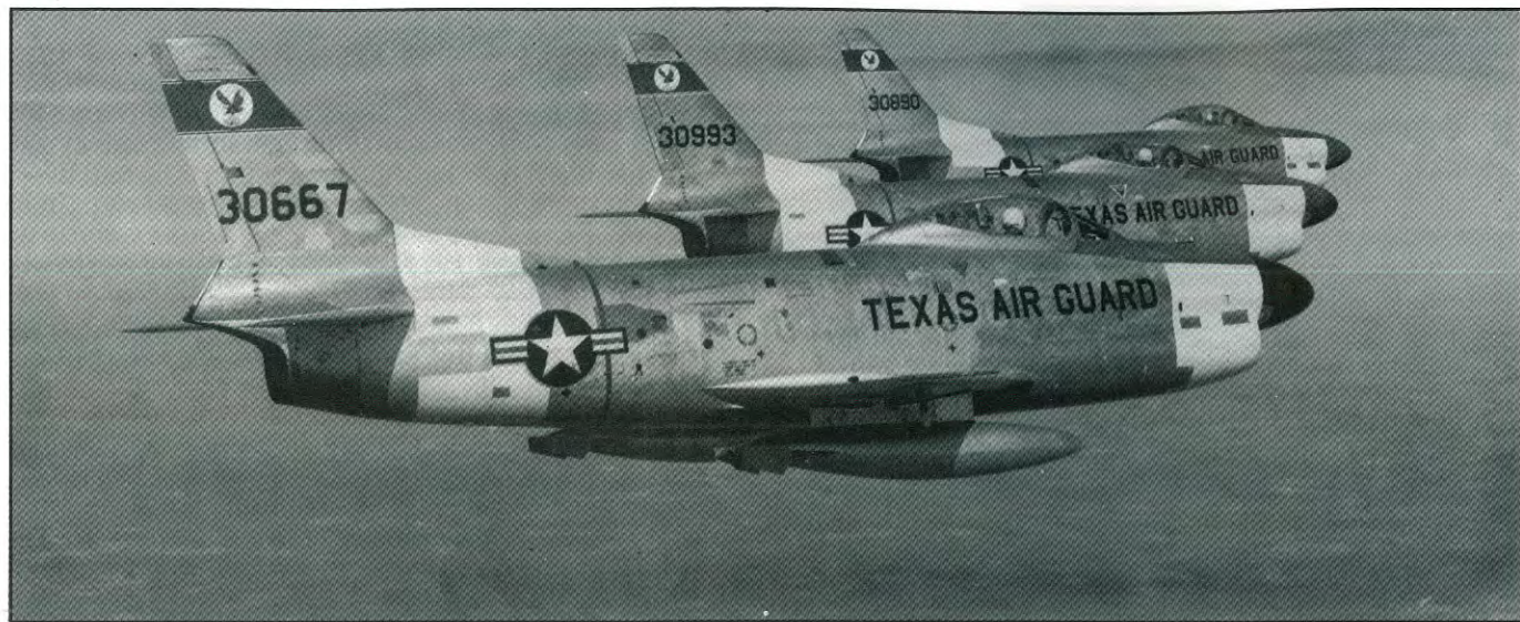
A trio of 182nd Squadron F-86Ls over Texas in 1959. The white areas on the fuselage are Day-Glo Red paint, applied to all aircraft as an air to air visibility aid. (credit - Larry Davis Collection)
