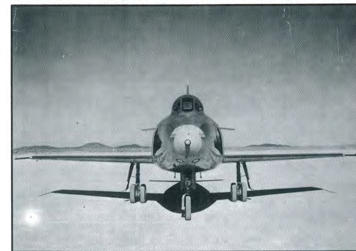
Looking 'down the throat' of the YF-93A, showing the recessed air intakes and fuselage shape. Within the nose radome was an SCR-720 Search Radar. (credit - NAA)
