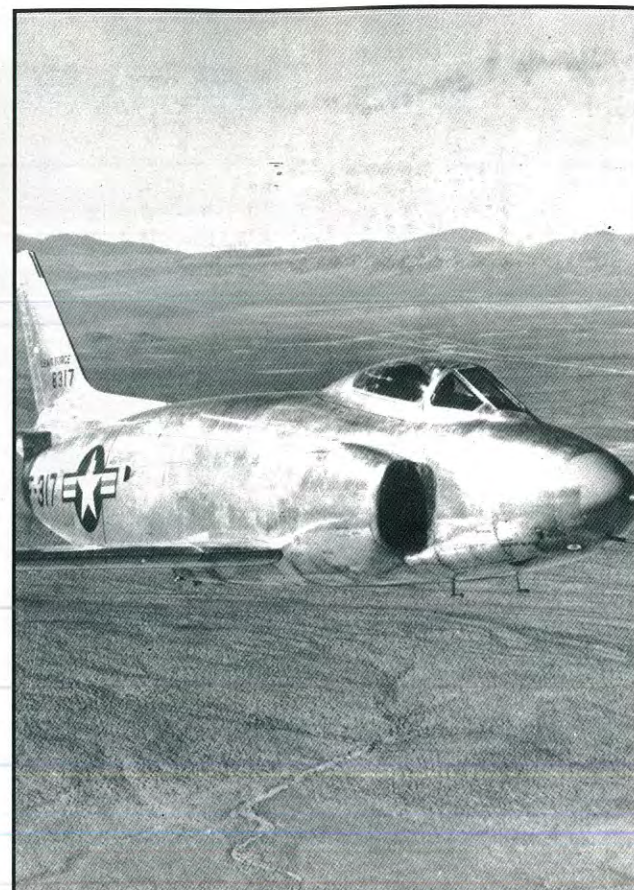
Inflight over Southern California, the first YF-93A has had the redesigned air intakes fitted over top of the recessed units. Air Force declined to purchase the YF-93A when SAC indicated the new B-47 was so fast it wouldn't need an escort fighter! (credit - NAA)
