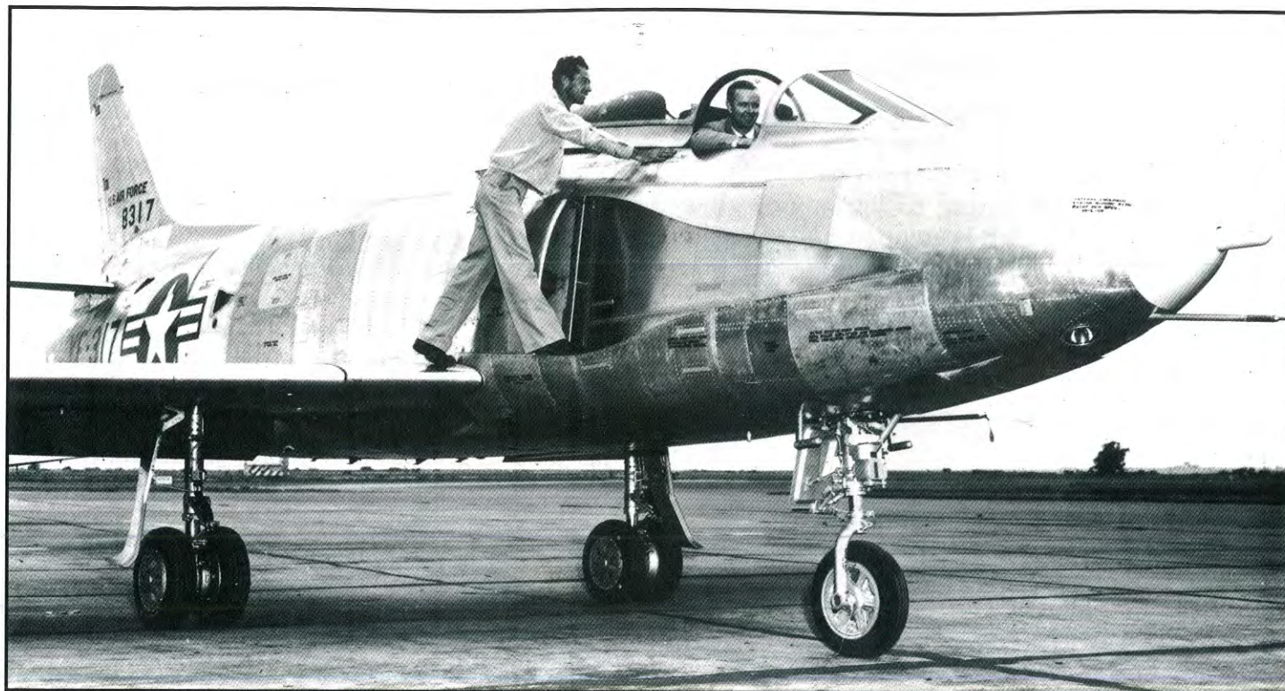
Two North American Aviation personnel make final checks to the first F-86C prior to its first flight on 24 January 1950. The radical NACA-designed recessed air intakes are very evident in this photo. (credit - NAA)
