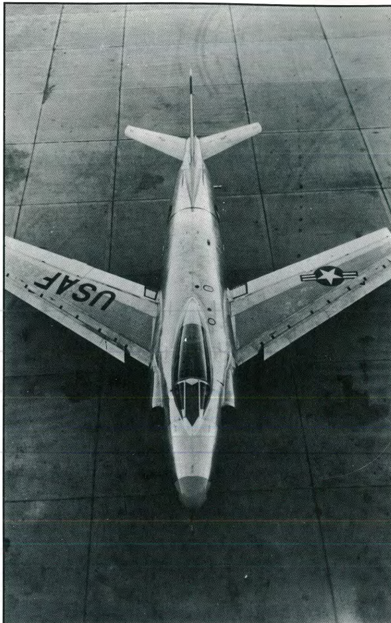
High front view of the no. 2 YF-93A, #48-318, which had standard air intakes installed over the recessed units found on the first airplane. Note the V-shaped windscreen originally used on the F-86A. (credit - NAA)
