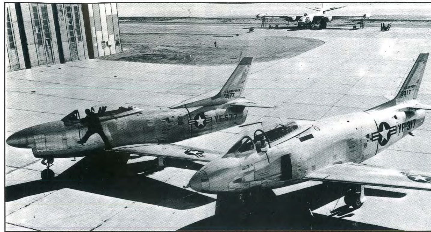
The newly designated YF-93A (ex-F-86C) shares the ramp at Muroc with the new YF-95A (F-86D) prototype. Both aircraft share various parts with the original F-86A Sabre, such as the windscreen and canopy, vertical and horizontal tail surfaces, and basic wing structure. (credit - NAA)
